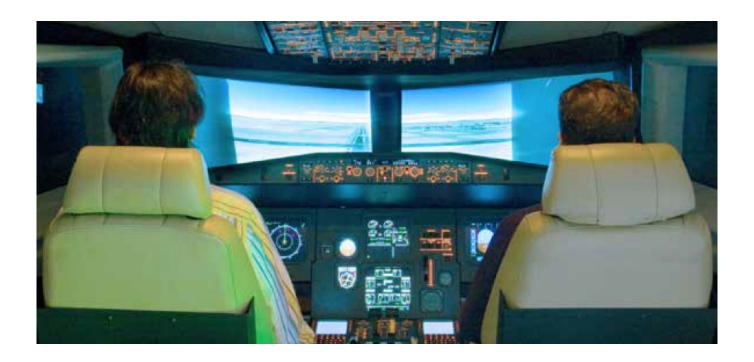
AACS is a cockpit simulator specifically designed for the ground validation of all area navigation (RNAV) procedures, for assessing the workload of a flight crew in nominal operation and in the case of contingencies, and for research in the area of cockpit human-machine interfaces.
